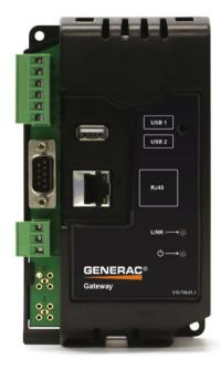
The Power Zone® Connectivity Gateway is a user interface for the Power Zone® system that provides external communication via ethernet to a connected device such as a computer, smart phone or tablet. This external communication allows the user to configure or monitor generator parameters, including building management system connections.
