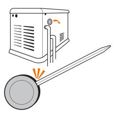
2. Locate and remove the gray plug on the back of your Home Standby Generator. If you have trouble, use the supplied wedge to loosen.
